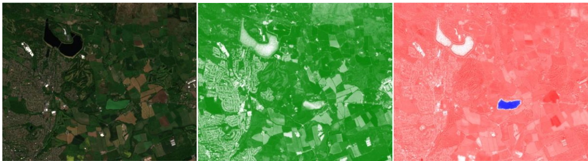
Figure 5: (Left) True colour, (Centre) Normalised Difference Vegetation Index and (Right) Normalised Mean Difference Water Index from Sentinel
